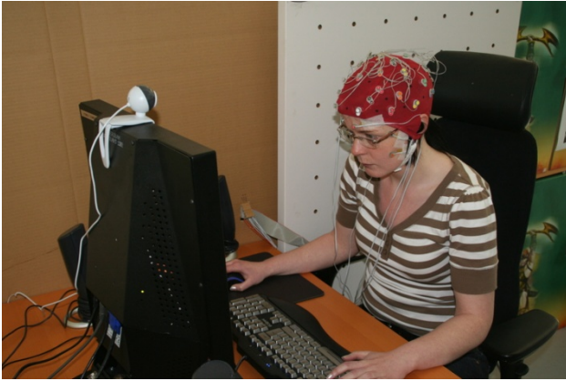
Figure 1: The eye-tracking screen, EMG sensors and electroencephalography array
