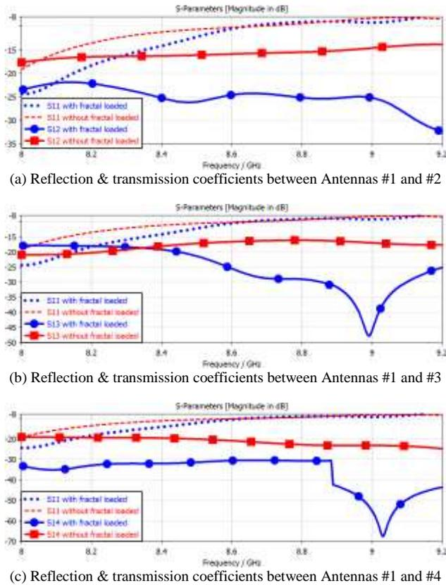
Fig. 2. Simulated reflection & transmission coefficients of the equivalent model for the proposed fractal structure.
