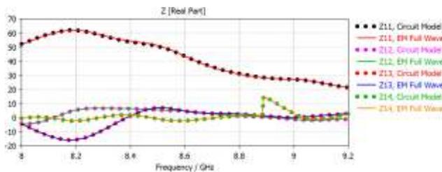
equivalent circuit model was used to determine the effectiveness of the fractal load on the antenna array's return-loss and isolation performance. Input impedance and admittance of the proposed antenna arrays computed using full-wave EM simulation tool are shown in Figs. 5. Due to the symmetrical configuration of the antenna array and accurate estimation of the  $RLC$  parameters the circuit model and CST results are perfectly mapped on each other for both of input impedance and admittance.
