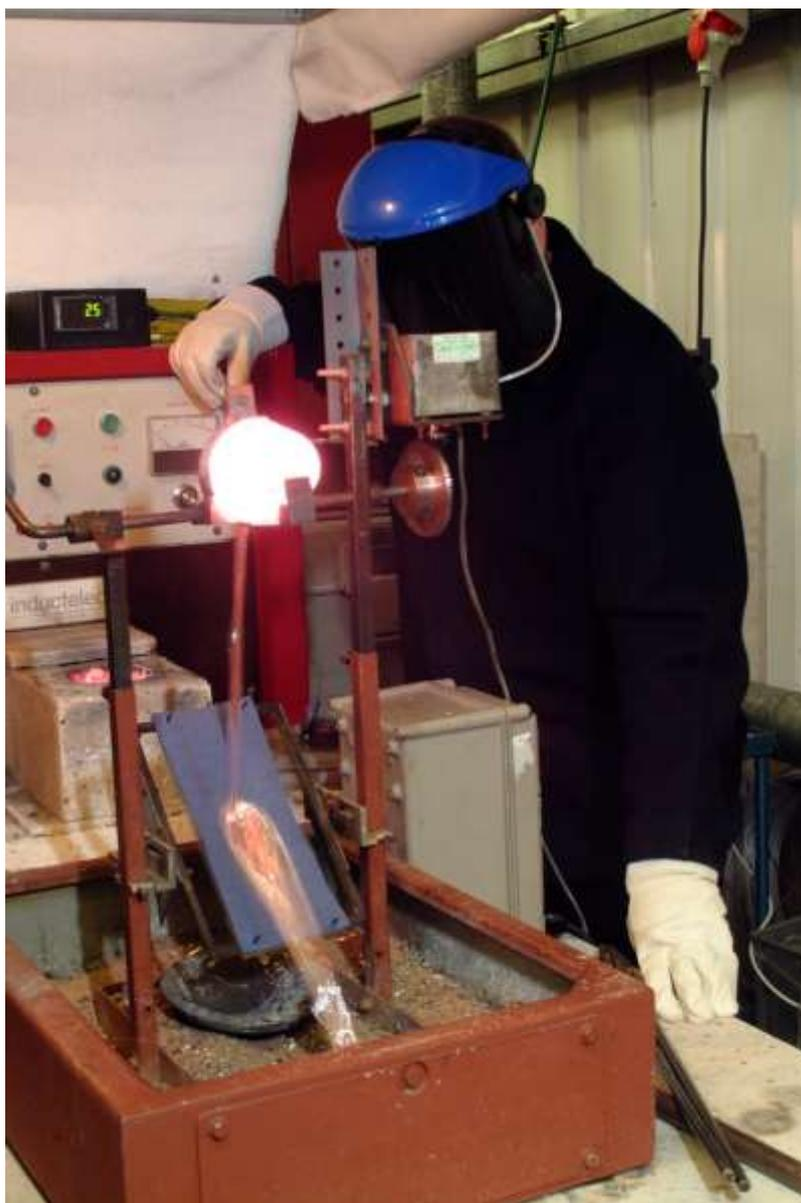
**Figure 3.7.** The hot metal splash test, BS EN ISO 9185:2007 (replaces BS EN 373:1993)
