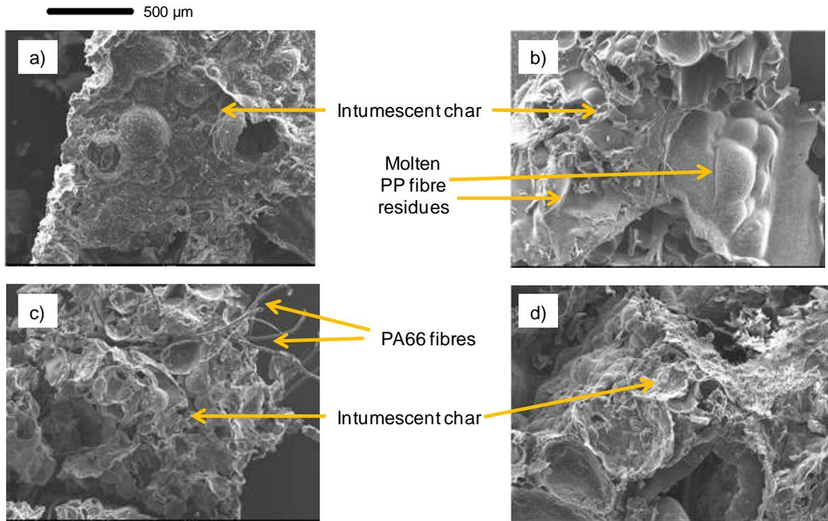
**Figure 5.** SEM images of intumescent foams of (a) PS-A silicate only and containing (b) PP nonwoven web, (c) PA66 nonwoven and (d) ARG woven mesh
