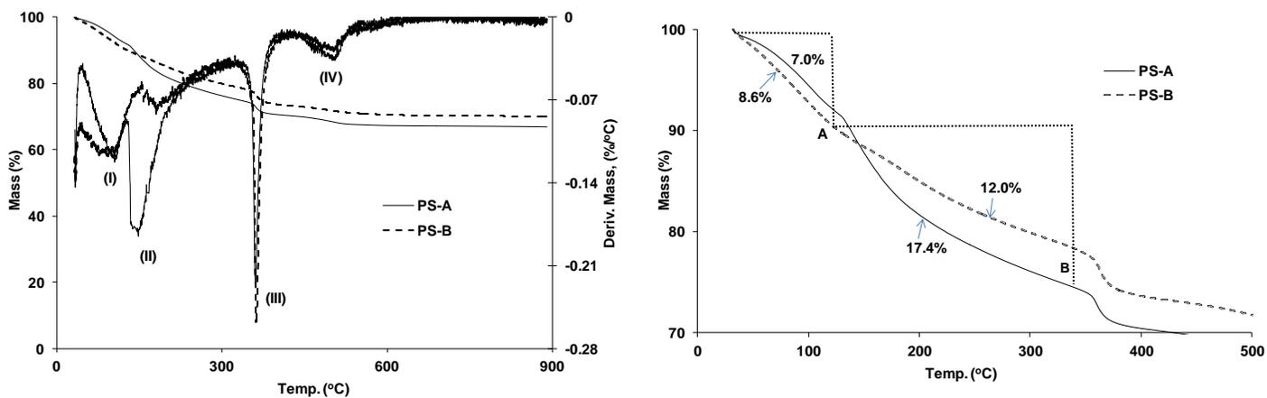
**Figure 3.** a) TGA – DTG curves of PS-A and PS-B silicate samples in nitrogen; b) mass loss from TGA curves in the temperature range RT–330°C.
