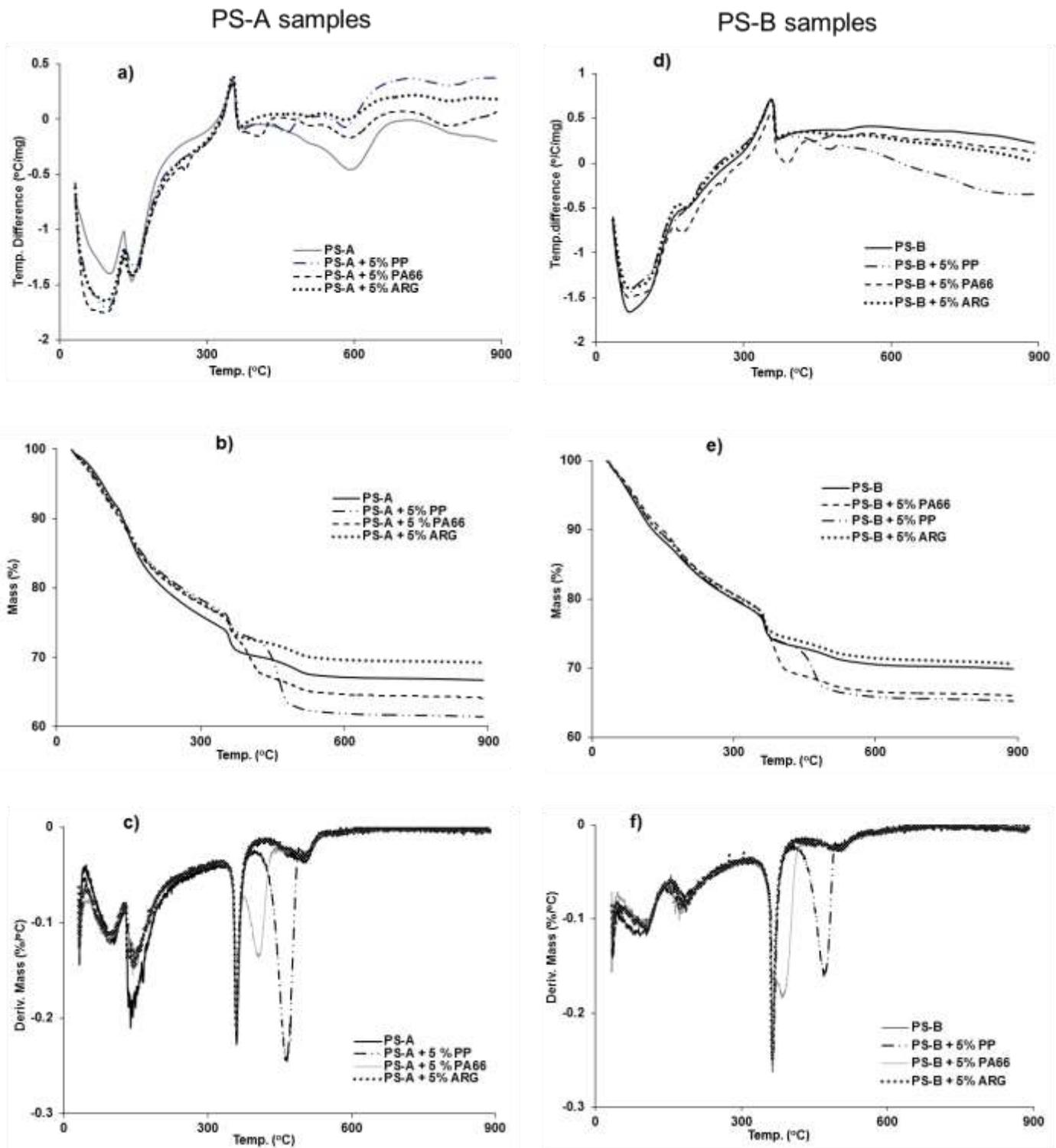
**Figure 2.** (a,d) DTA, (b,e) TGA and (c,f) DTG responses in nitrogen of PS-A (a-c) and PS-B (d-f) silicates with 5% PA 66, PP and ARG fibres.
