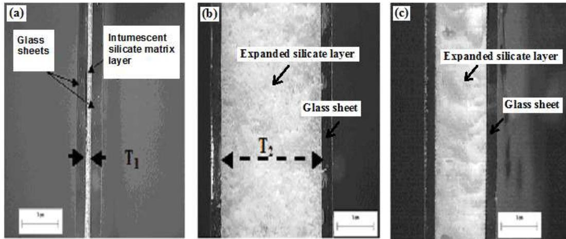
**Figure 1.** (a) Glass-silicate-glass composites; expansion of silicate layers under thermal shock: (b) PS-A and (c) PS-B.
