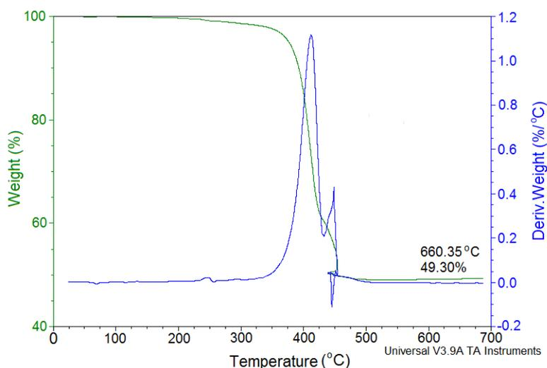
**Figure I.** TGA Analysis of Stainless Steel Fibre
