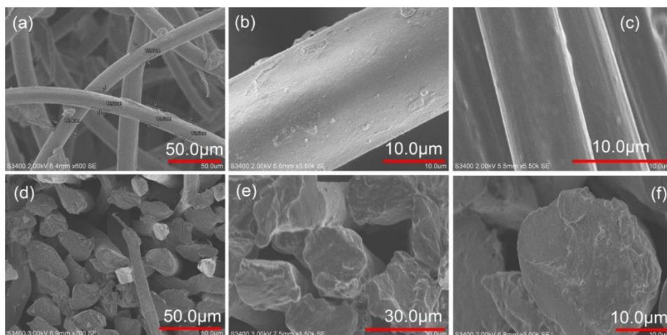
**Figure II.** SEM (a, b) Longitudinal Images of Stainless Steel and (c) Carbon Fibres and (d, e, f) Cross-Sectional Images of Stainless Steel Fibre
