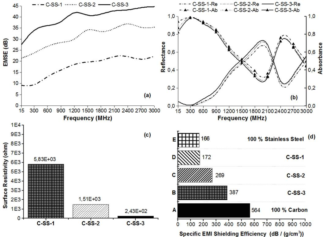
**Figure V.** (a) EMI Shielding Efficiency of Needle Punched Nonwoven Fabrics with Different Percentage of Carbon Fibres between 15MHz and 3000MHz. (b) Absorbance and Reflectance Results of Needle Punched Nonwoven Fabrics with Different Percentage of Carbon Fibres between 15MHz and 3000MHz. (c) Surface Resistivity Results for Needle Punched Nonwoven Fabrics. (d) The Comparative of Specific EMI Shielding Efficiency of Our Data with Other Reported Results
