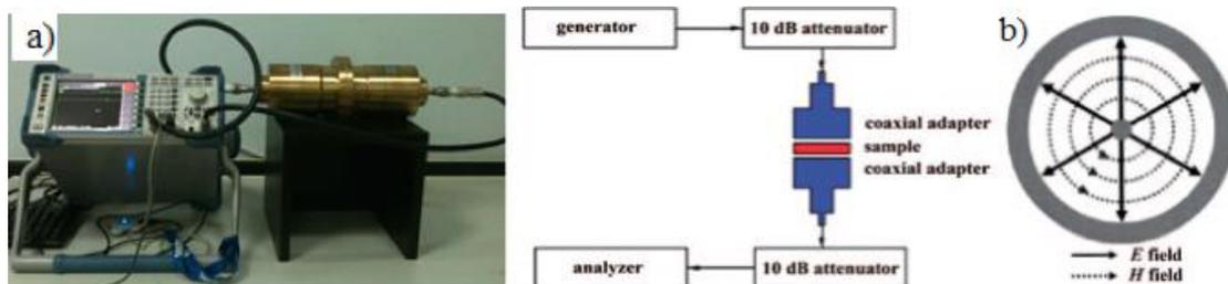
**Figure IV.** (a) Set-up with coaxial adapters (b) electric (E) and magnetic (H) field distribution inside a coaxial line [8]
